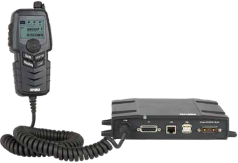
Cobham Explorer Mobile Gateway: A durable, dual-mode handset with a reinforced push-to-talk button and a high audio loudspeaker to deliver fast and simple communications
